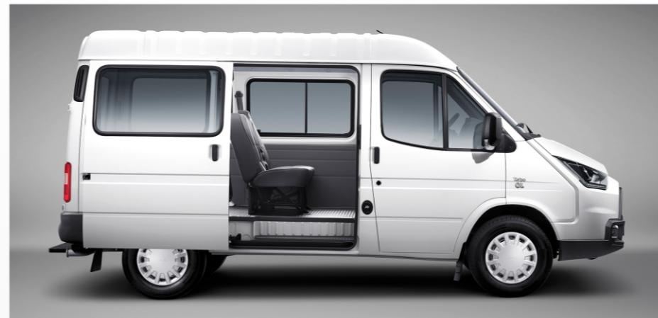
All models with 1100mm open width side door make loading more convenient
